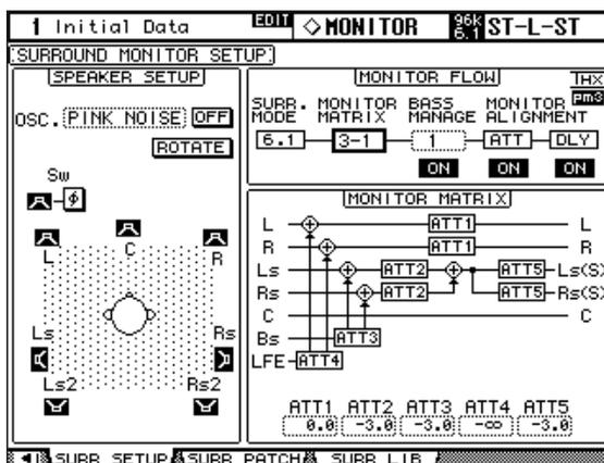
**2 Use the cursor buttons to select the parameters, and use the Parameter wheel, INC/DEC buttons, and [ENTER] button to set them.**
