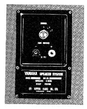
Rotary switch type tone control incorporated. Under ordinary circumstances, set at NORMAL. If the high frequency response is too strong, reduce it by setting the switch to "1" or (for greater damping) "2."
