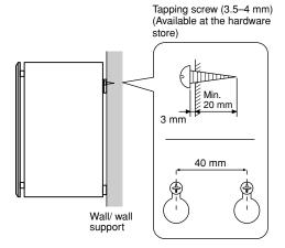
You can also use the screw holes on the rear of the speaker for installing the speaker using a commercially available speaker bracket (if you do not use the attached mounting bracket).
