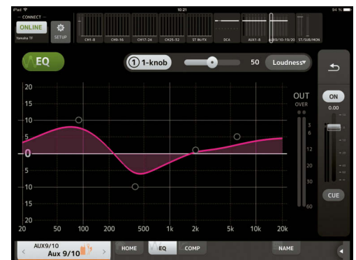
1-knob mode adjustments for parametric EQ in the outputs set to “Loudness” (figure 21)
