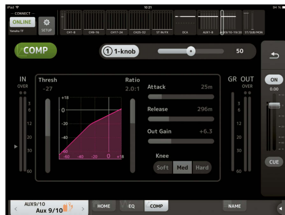
Compressor 1-knob adjustment for quick access without irritating or confusing beginners (figure 23)
