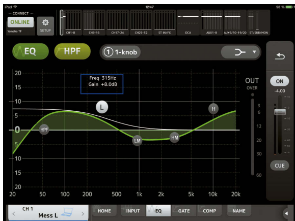
Parametric EQs in all inputs fully equipped, alternatively the EQ can be set to “1-knob” mode (figure 14)
